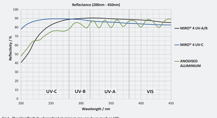
Fig.1 - The UV reflectivity of anodised aluminium can vary by as much as 10%
