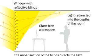
The upper section of the blinds directs the light into the depth of the room. The lower section enables glare-free light redirection to the ceiling.
